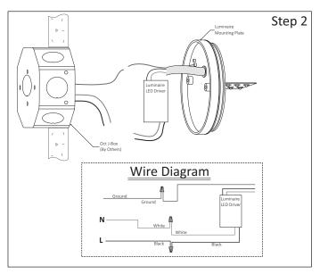
Step 2 - Make Wiring Connections:
