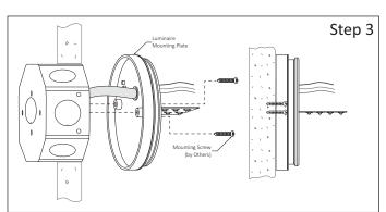
**Step 3** - Install Luminaire Mounting Plate:
