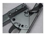
Place fast pins in position as shown above. Top pin will be always as shown. Bottom pin can be used in alternate positions to adjust angle. For the closest to 90 degree place pin in bracket as shown below and allow tier arm to rest on pin.
