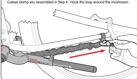
Note: If more spring tension is needed, tie a knot in the static cord, but leave room for the loop to attach to the mushroom assembly.
