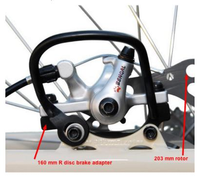
NOTE: Avid has recently (as of 2012) made minor changes to rotor sizes (203 mm rotor became a 200 mm rotor for instance). For best results, we recommend following the recommendations above exactly - don't use the new Avid rotor standards, for risk of mis-aligned disc brakes.
