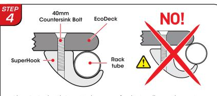
Place EcoDeck with SuperHooks on top of racks. Install one side at a time. Twist SuperHooks so that they are aligned with and snug to racks. Once SuperHooks are in proper place, tighten one side until firmly secure. With one side complete, repeat on other side. If the rack distance is too wide, refer to **Step 2** above to squeeze them together until SuperHooks are completely under the rack. Tighten SuperHooks bolts and remove CamStrap or belt when finished. DO NOT pinch rack with SuperHook
