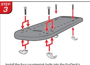
Install the four countersink bolts into the EcoDeck's countersunk holes. Screw bolts into SuperHooks a couple turns so that they're on, but loose. The forward hook positions have two options for install, but we recommend using the forward most holes.
