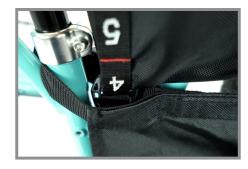
**Note:** If using a Sling over a CargoBay on an EdgeRunner or LEAP, buckle the Sling to the frame upright, outside the vertical webbing that connects the CargoBay to the "chainstay" of the EdgeRunner or LEAP.
