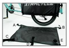
Place one Sling facedown. Xtracycle logo should be facing the floor and away from you with the Sling mounting side-release buckles A & B closest to the bike.
