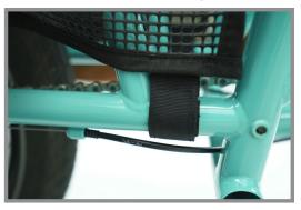
Attach hook-and-loop straps to the horizontal "chainstay" tube at the bottom of the EdgeRunner frame. Pull each strap tight before securing. Be careful to not wrap webbing around housing or cable.
