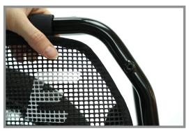
The angle of the WheelSkirts will match the angle of the V-Rack with the Xtracycle logo facing out.
