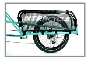
Go back and tighten all straps until WheelSkirt is firmly tensioned around the rack and bottom of frame. Pressing with your hand toward the wheel with ten pounds force you should not be able to cause the WheelSkirt to touch the tire.
