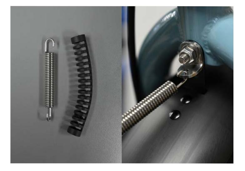
Using an 8mm box wrench loosen the nyloc nut and unscrew the eyelet bolt and L-bracket.
