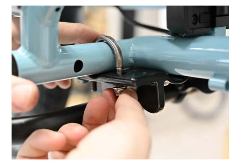
Place the second U-Bolt on the non-drive side and position the small mounting mounting plate in place on the forward threads. Secure it with an M6 washer and nut.
