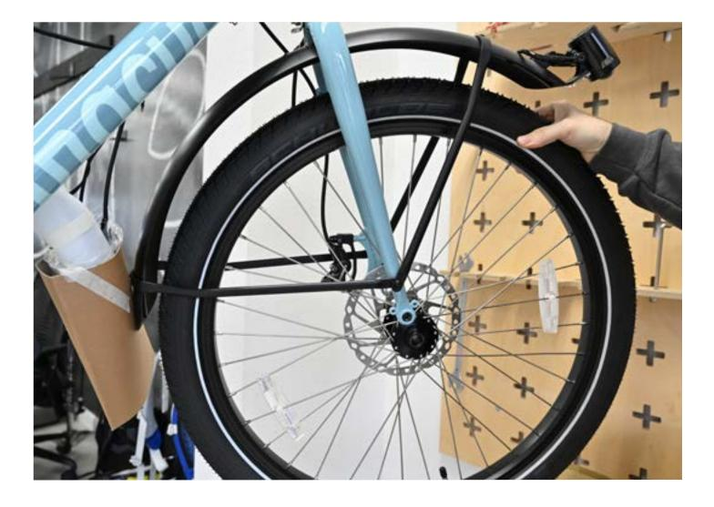
Re-insert your thru-axel, and tighten with a 6 mm Allen wrench.
