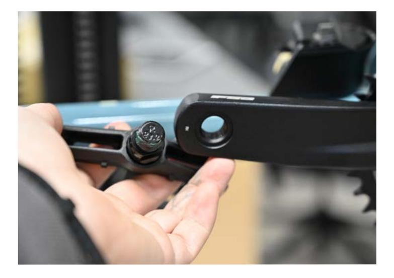
With the right pedal, start threading the pedal bolt into the crank arm. Once initially threaded you can backpedal while holding the pedal bolt in place. The left pedal has a reverse thread so you will need to turn the pedal bolt counter clockwise to tighten it.
