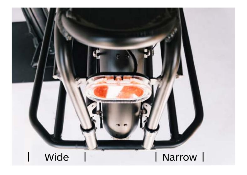
If you would like to switch the width setting on your U-Tubes to narrow or wide: Press the spring pin button in and push or pull the spring pin elbow on the inside of the U-Tube until the button pops through the width setting hole you desire. Needlenose pliers might be needed to help with this.
