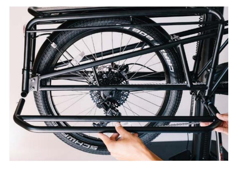
If your U-tubes do not seem to easily slide into the frame, you will need to loosen the tailpiece on the back end of the bike in order to acquire additional tolerance. This is the tail piece.
