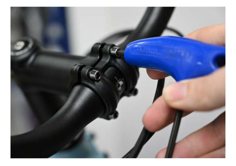
Use a 3 mm Allen wrench to loosen the paddle grips. Reposition them so they are level with the ground. Then retighten them.
