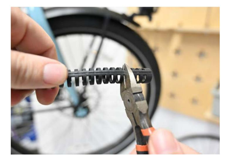
Slide the spring sleeve over the Stabilizer Spring.
