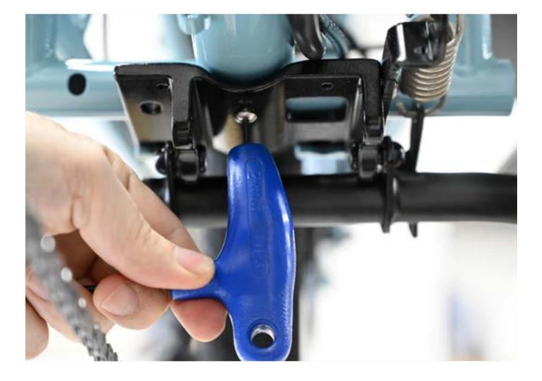
Install the first U-bolt on the drive side of the bike. Fit an M6 washer and nut onto the forward threads, until just finger-tight. Place a nut on the other end of the U-bolt, and secure to finger tight.
