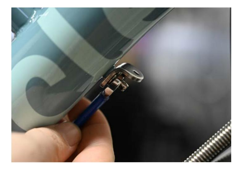
Replace the eyelet bolt and nyloc nut. Keep the nyloc nut a bit loose so that you can rotate the eyelet bolt.
