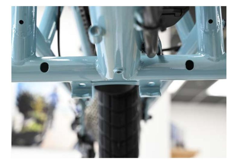
Rest the back of the kickstand mounting plate on the mounting shelf and use a 3 mm Allen wrench to thread the M5 set screw in order to hold the kickstand in place.
