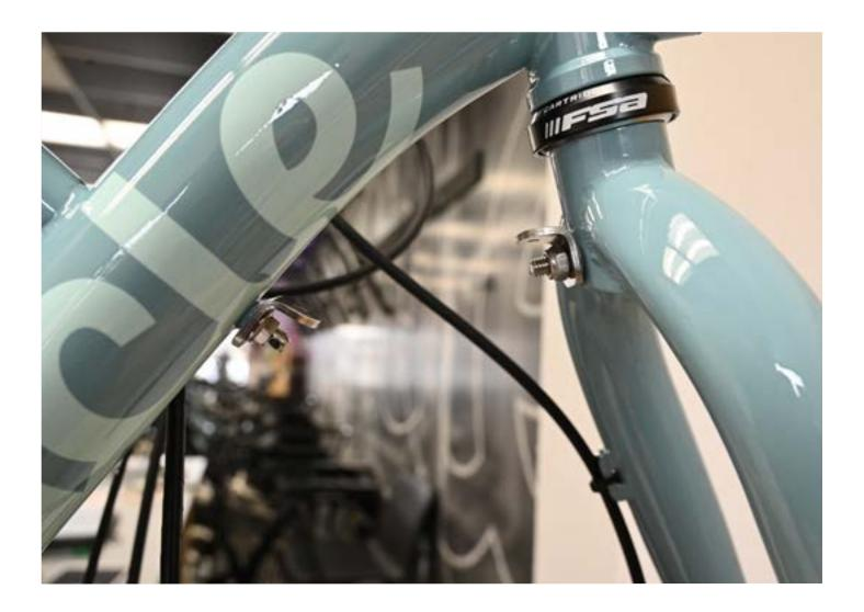
Bring the front fender into position by hanging the mounting tab from the M6 x 50 mm bolt, followed by the L-bracket, & M6 washer, holding it in place with the M6 nyloc nut. Keep secure, though you will tighten this in a moment.
