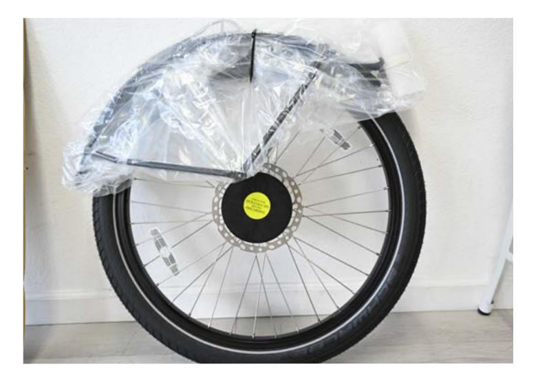
Remove the packaging around the fork and fender. Remove the thru-axel with a 6 mm Allen wrench.
