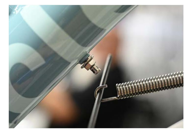
Using an 8mm box wrench tighten down and secure the nyloc nut.
