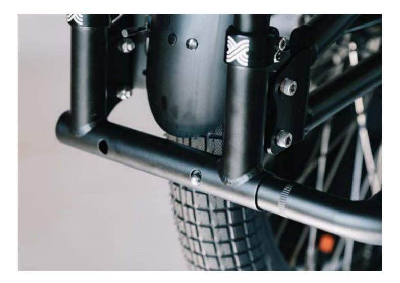
Insert the remaining U-Tube on the other side of the frame.
