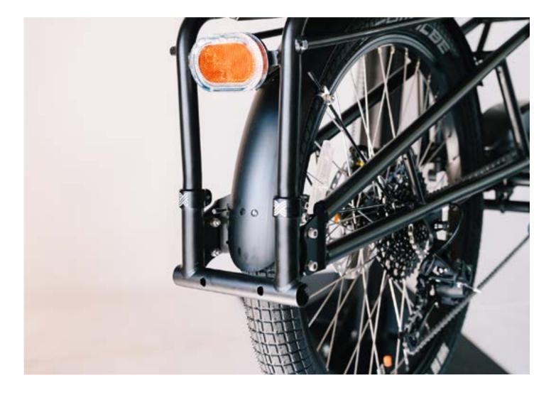
Four bolts secure the tailpiece in place. Loosen these four bolts using a 10 mm wrench and a 5 mm Allen wrench.
