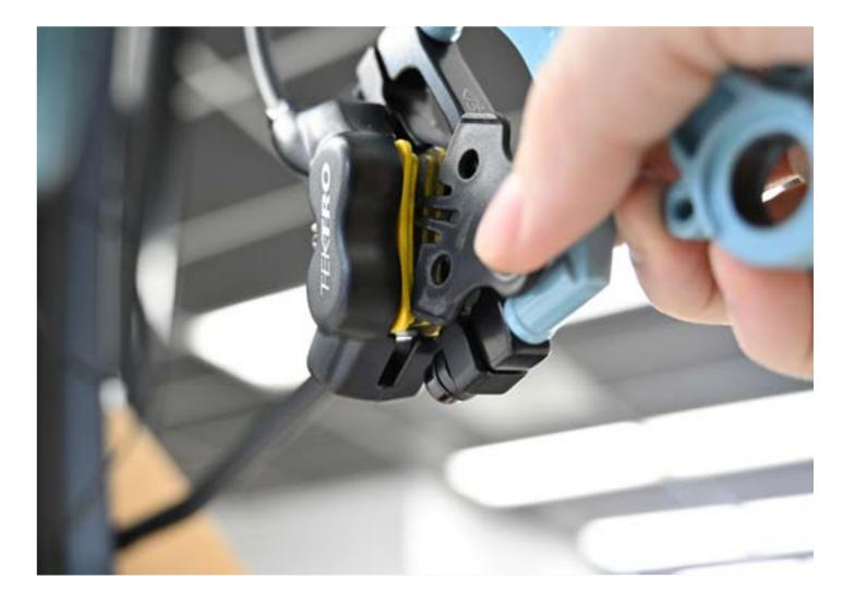
Rotate your front wheel into position. Be mindful to seat the disc brake rotor neatly between the brake pads.
