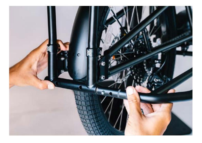
Insert the U-tube into the frame, pushing in on the spring pin button so that the button slides into the frame as well. Insert the U-tube far enough for the spring pin to pop out into the hole on the bike frame.
