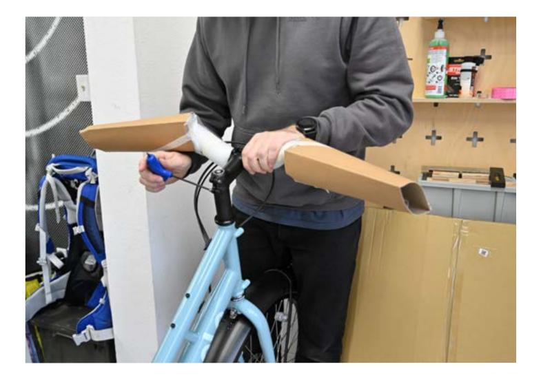
Use a 4 mm Allen to loosen the faceplate on the front of your stem, and center the registration marks and angle the bars in a vertical position that is most comfortable for you. Then retighten the faceplate.
