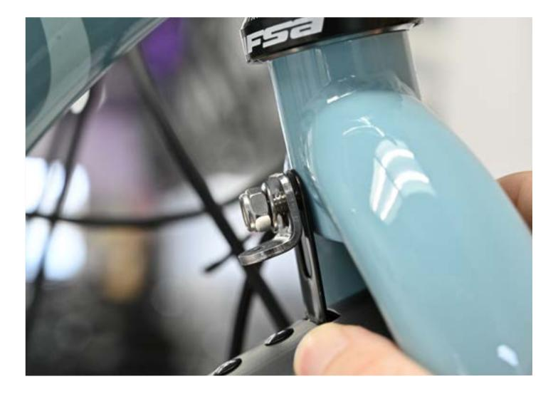
Use a 3 mm Allen wrench to attach the outer support arms of the fender to the lower fork-mounting points with the two M5 bolts.
