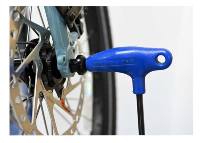
Returning to the fender, tighten the upper bolt with a 4 mm Allen wrench and an 8 mm socket tool.
