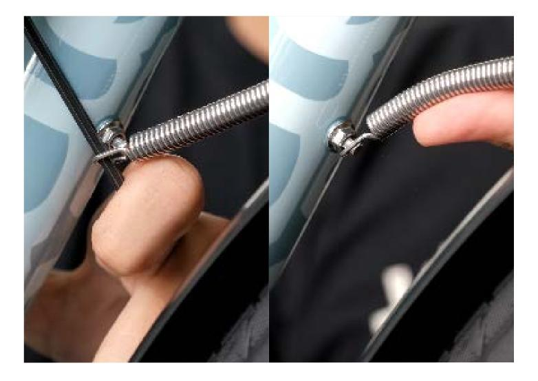
Slide the spring sleeve over the StabilizerSpring.
