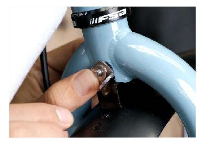
Usa a 4 mm Allen wrench to attach the outer support arms of the fender to the lower fork-mounting points with the two M5 bolts.
