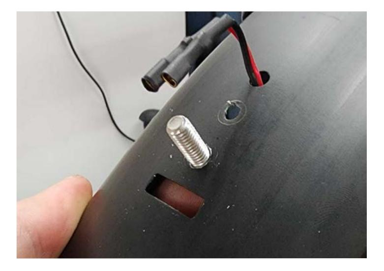
Once the light is secure you're going to connect the spade connectors (from fender to light - red to black; black to black with gray stripe).
