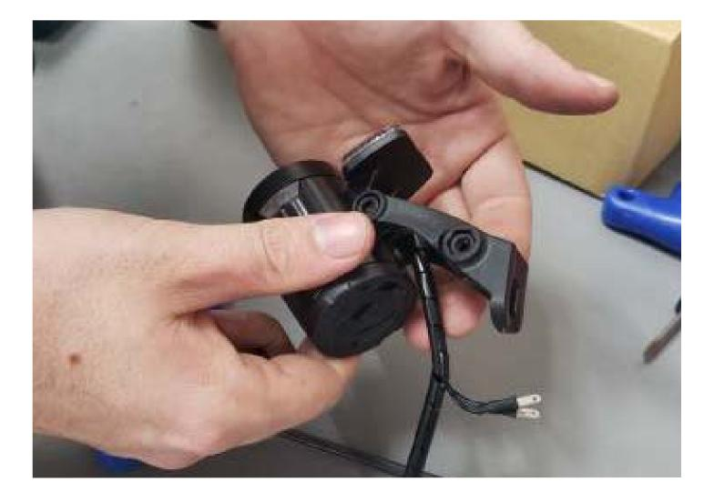
Insert the M6 bolt through the forward most hole on the fender to attach the front light. Using an M6 nyloc nut and a 5mm Allen wrench secure the light to the fender.
