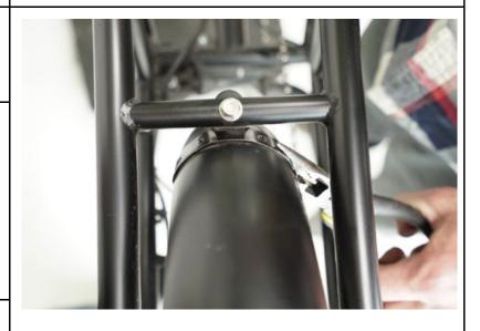
Check the clearance between the chain and front of the rear fender when in the lowest gear combination (biggest rear cog and smallest front chainring). If the chain is too close to the fender, it may get caught on the fender while pedaling.
