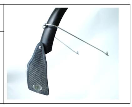
Attach the riveted on L-bracket at the top of the front fender to the crown of the fork with the the M6X55mm bolt, in the configuration shown.
