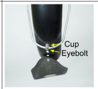
Like the u-shaped stay, the straight rear fender stay mounts to the hole on the front of the fender with an eyebolt, cup, and M5 nyloc nut.
