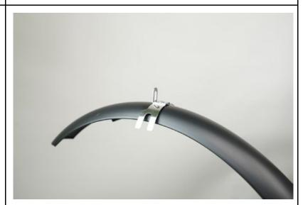
Bolt the bridge mount to the seatstay bridge using the M6x25mm bolt and nut.
