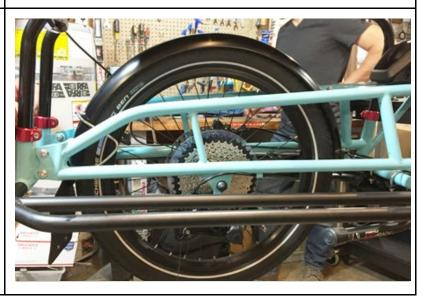
Once the fender is aligned, use an 8mm wrench to tighten both of the M5 nyloc nuts holding the eyebolts, making sure the nyloc is fully engaged. (you may find it easier to temporarily remove the rear wheel to access these nuts).
