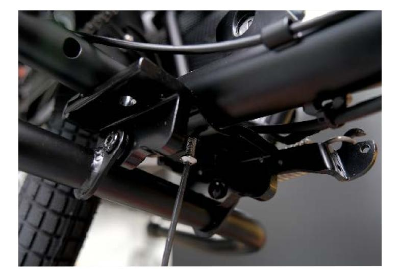
Install the first U-bolt on the drive side of the bike. Fit an M6 washer and nut onto the forward threads, until just finger-tight.
