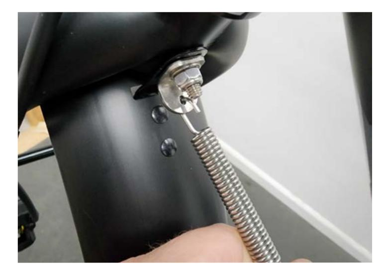
Use an Allen wrench or screwdriver to pull the other end through the eye-bolt.
