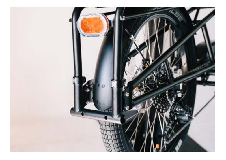
Push or pull the tailpiece into a place where you can easily insert the U-tube.
