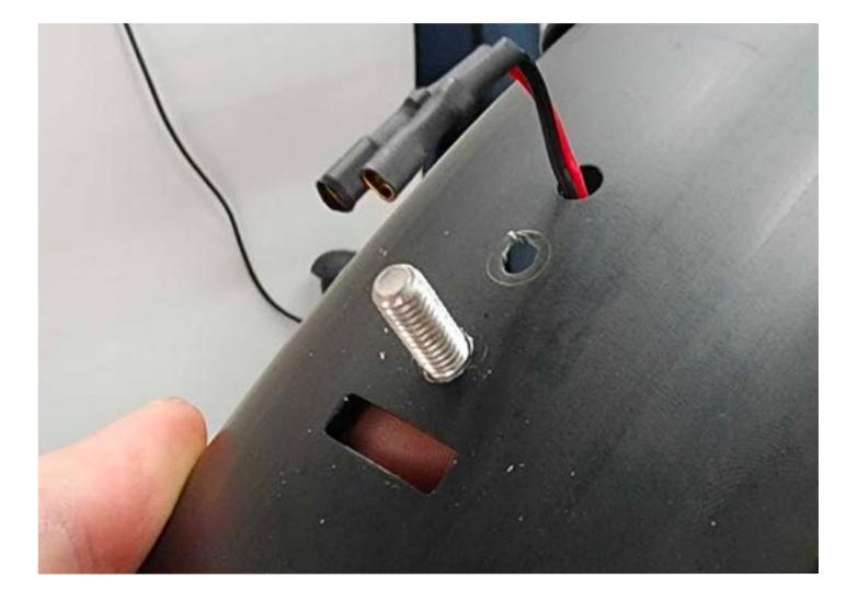
Before you mount the light to the fender you should flip/rotate the piece of the light mount that attaches to the fender to look like the image here.
