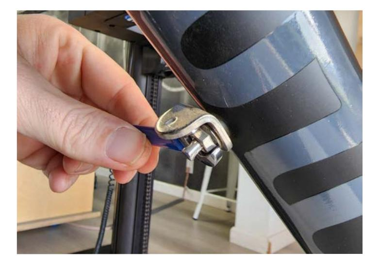
Hook the StabilizerSpring to the L-bracket on the fork.
