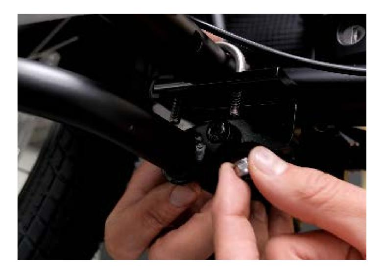
Place the second U-Bolt on the non-drive side and position the small mounting mounting plate in place on the forward threads.
