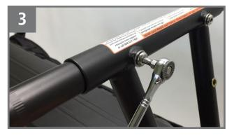
Tighten the M5 bolts using a 4mm Allen key.
