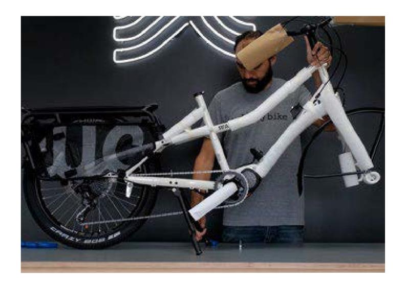
Remove the packaging around the fork and remove the thru-axel with a 6 mm Allen wrench.
