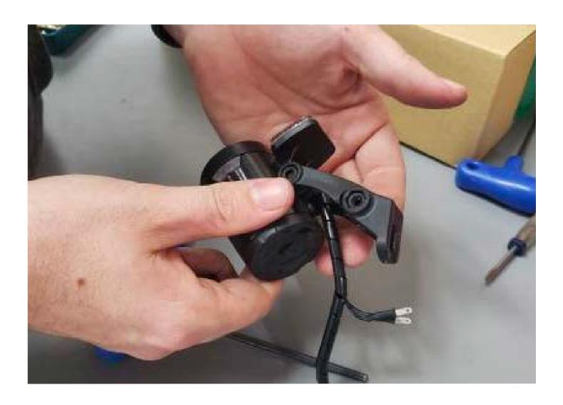
Now you'll attach the light mount to the M6 bolt in the fender and secure with an M6 nyloc nut. Use a 5mm Allen wrench from the underside of the fender to tighten the bolt and nut securing your front light to your fender.
