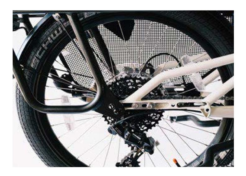
Position the FootRest on the bike and loosely thread the two 8 mm bolts through the front mounting plate and into the threads on the frame. You may need an extra hand to help hold up the UtilityRack while you thread in these bolts. The bottom portion of the rear clamp should fall underneath the UtilityRack.
