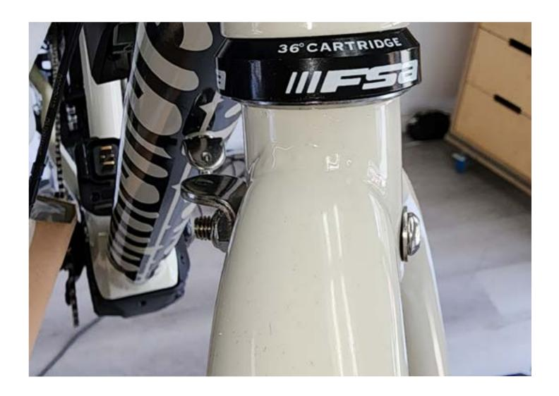
Install your fender using the M6 bolt already in the fork. The order should be fender tab, L-bracket, washer, M6 nyloc.
