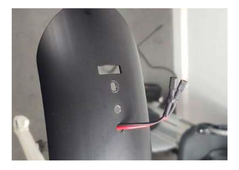
You will be attaching the light through the forward-most rivet hole. To receive the bolt, you can either drill out that hole a little bigger or use the bolt to open it up a little. Insert M6 bolt through the hole.
