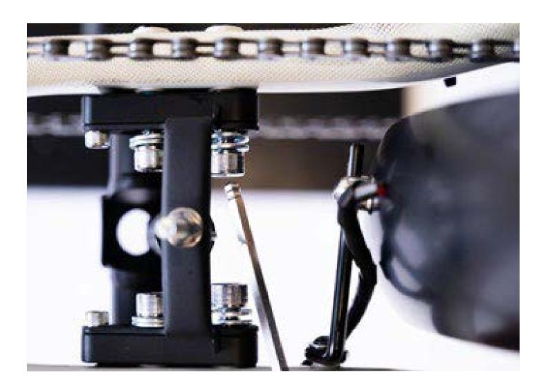
Using the shorter end of the Allen wrench, tightly secure all bolts in place.
