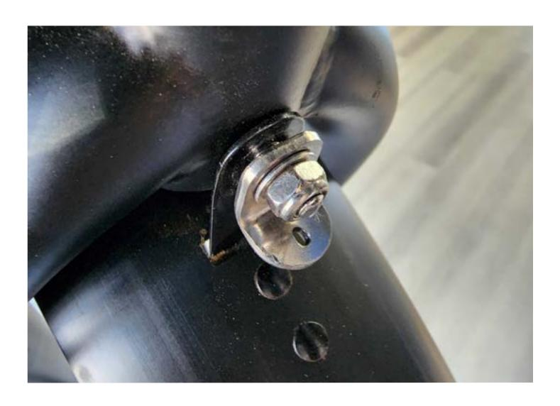
Usa a 4 mm Allen wrench to attach the outer support arms of the fender to the lower forkmounting points with the two M5 bolts.
