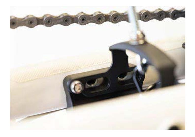
Place two washers on one of the M8 bolts. Starting on the inside of the mounting plate and using just your fingers, thread the bolt with the washers to the front boss until you can not turn it any further. You should be able to thread the bolt until you are certain it has engaged with the threaded boss on the chainstay.
