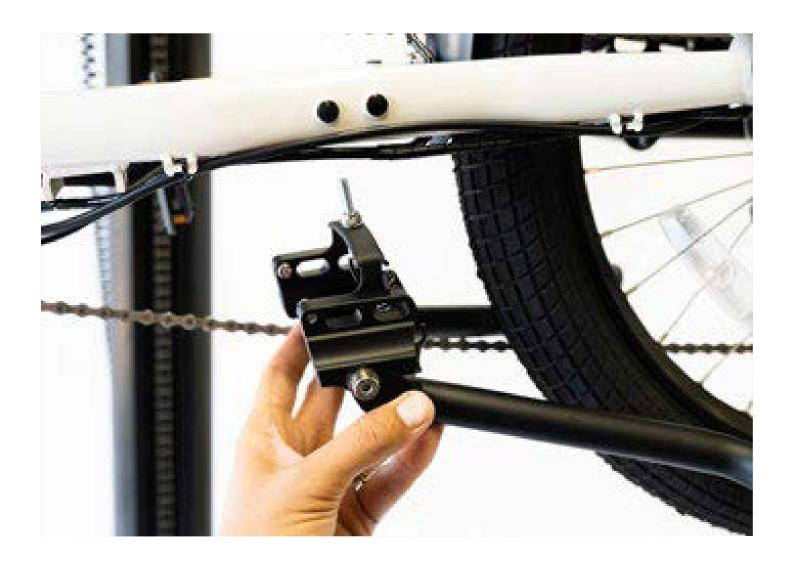
Place the KickBack so that the 2 ovalized holes on each side line up with the bosses on the inside of the chain stay.
