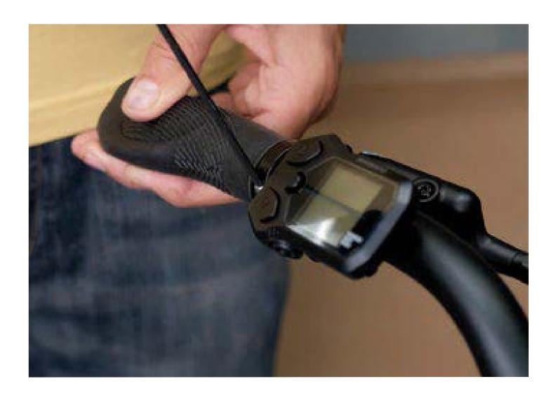
Use the provided Shimano lead-connector tool from the small parts box to insert the display cable into the small port under the display. You should feel a securing click when the connection is made.
