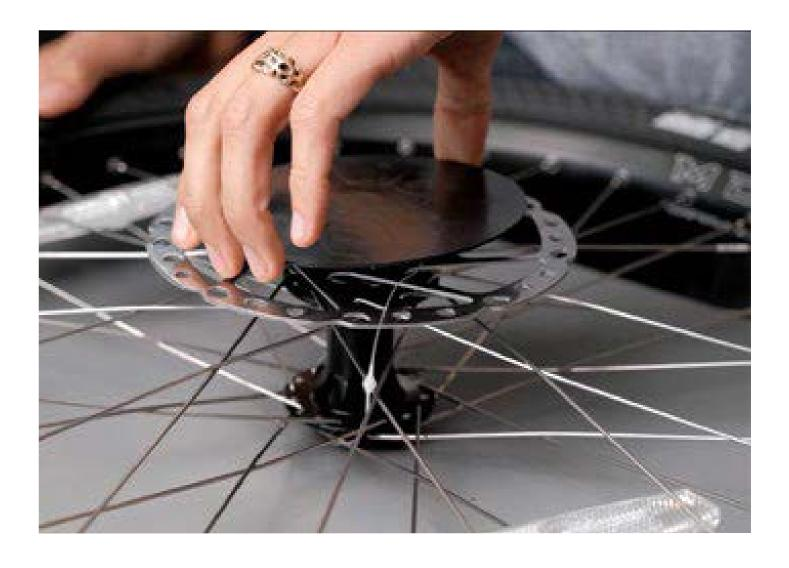
Double check that the drive side hub cap on your wheel isn't stuck to the plastic disc packaging.
