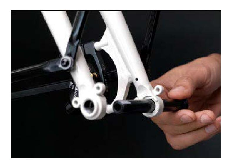
The hardware for you fender is already installed in your fork. Please remove the M6 nyloc nut and L-bracket.
