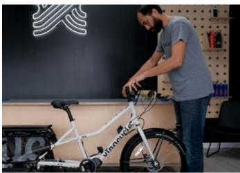
Use a 4 mm Allen to loosen the faceplate on the front of your stem, and center the positioning target. Then retighten the faceplate.
