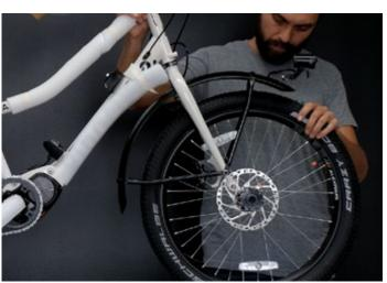
Re-insert your thru-axel, and tighten with a 6 mm Allen wrench.
