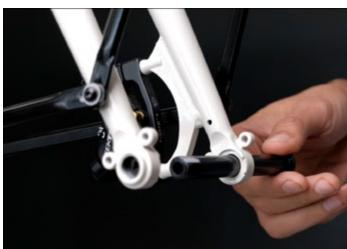
Remove the disc brake-pad spacer.
