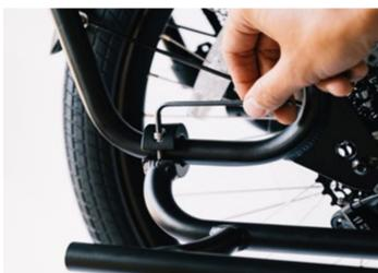
**48** Re-tighten the bolts securing the UtilityRack to the frame.
