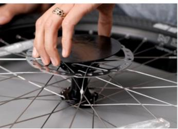
Rotate your front wheel into position. Be mindful to seat the disc brake rotor neatly between the brake pads.
