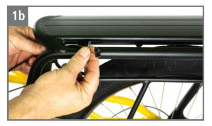
Remove the tail light cable from the Utility Rack and rear frame, snipping any zip ties holding it in place
