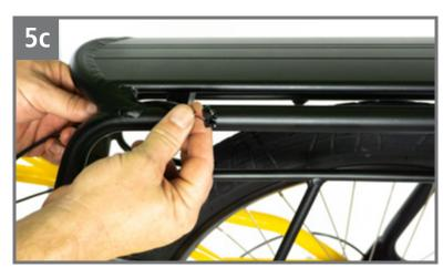
Feed the tail light cable along the inside of the non-drive side of the rack and use small zip ties to secure it in place
