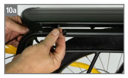
Feed the tail light cable along the inside of the non-drive side of the rack and use small zip ties to secure it in place
