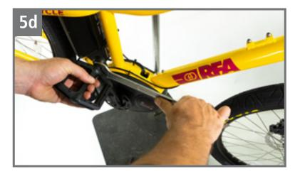
Grease threads and install left and right pedals
