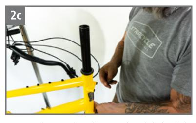
Grease the steer tube and insert up through the head tube
