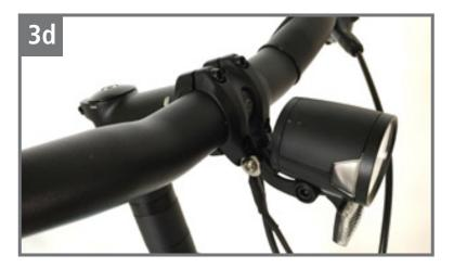
Install headlight with Allen key and 8mm open end wrench
