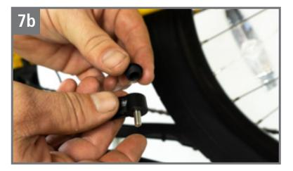
Remove the cap to the speed sensor and position it on the speed sensor post
