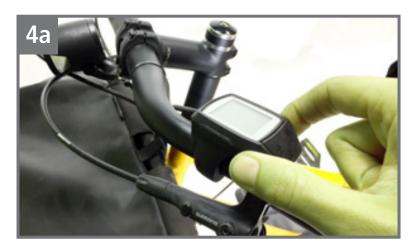
Mount Purion display to the left side of the handlebars, right of the brake lever
