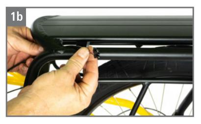
• Remove the tail light cable from the Sport Rack and rear frame, snipping any zip ties holding it in place
