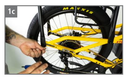
Remove the four bolts securing the Sport Rack using a 5mm Allen key
