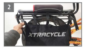
Select the RFA SlingSet with the complimentary buckle ends and connect to the buckle ends you just installed. Repeat steps for the opposite side.
