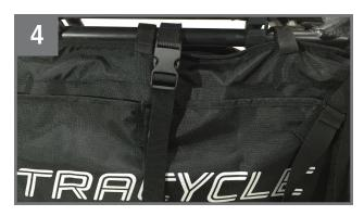
Optiona: If also installing a RFA CargoBay, wrap the attached hook & loop rings directly next to the RFA SlingSet buckles.
