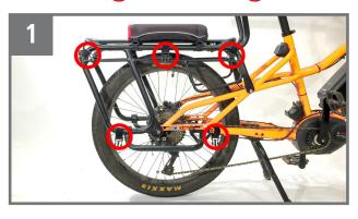
Attach three buckle ends to upper Utility Rack frame with the hook & loop rings. Attach the two remaining buckle ends to the lower rack and bike frames.
