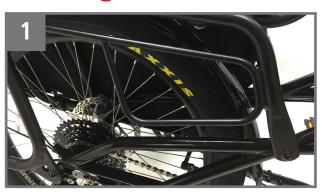
Loosen the two front bolts, and remove the two rear bolts that attach the Utility Rack to the RFA frame prior to starting.
