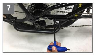
Check for proper threading on all bolts and alternatingly tighten each until the Footsie is secure.
