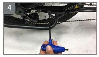
Align bolt positions on RFA Footsie with the threaded holes on RFA frame. Route the derailleur cables behind the RFA Footsie front mounting plate. Do not pinch cables. Loosely thread the front two M8 bolts.
