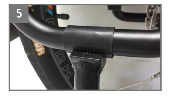
(Optional): Wrap a rubber pad around the Utility Rack at the point where the clamp assembly attaches. You will need to temporarily remove one of the front M8 bolts.
