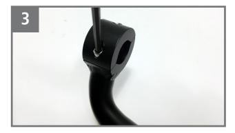
Remove the upper clamp assembly from drive side RFA Footsie.
