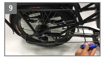
Thread the two rear bolts that connect the Utility Rack to the bicycle frame, then torque all four bolts to 30Nm with a 5mm Allen key.
