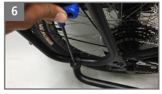
Place upper clamp assembly on the Utility Rack and loosely thread the M8 bolts.
