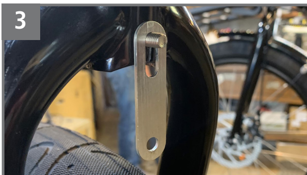
3 Install the fender/stabilizer bolt through the fork crown. The fender extension bracket should be installed with the long slot end up.
