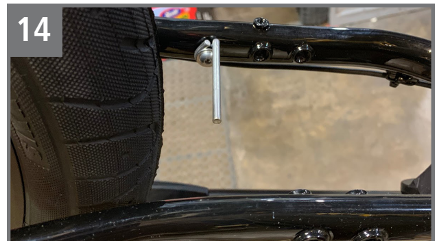
14 Utility mode requires use of the rear fender "lollipop" bracket set in the vertical position for optimal clearance. To increase clearance rotate clockwise.
