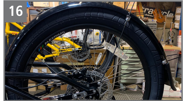
Loosen the strut nuts and push the struts through the brackets until the strut eyelet aligns with the fender boss on the sliding dropout insert.
