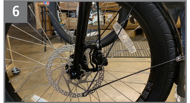
6 Loosen the strut nuts and push the struts through the brackets until the strut eyelet aligns with the fender boss on the fork blade.
