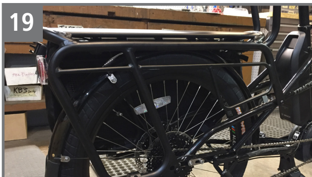
With your rear Fender installed you will now be able to install a rear rack.
