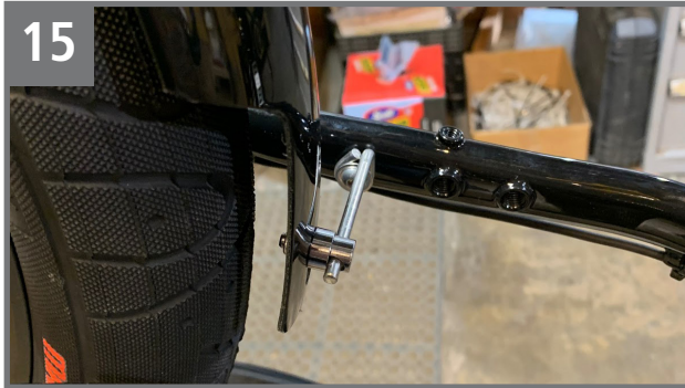
For Utility mode, Install the daruma cup and eye bolt on the fender first. Then feed the lollipop through the attachment hole and rest the Fender on the rear tire.
