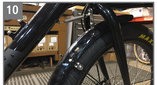
10 This is what the front Fender will look like once installed.
