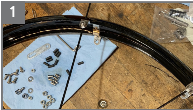
1 It is easier to assemble the Fender struts off the bike.
