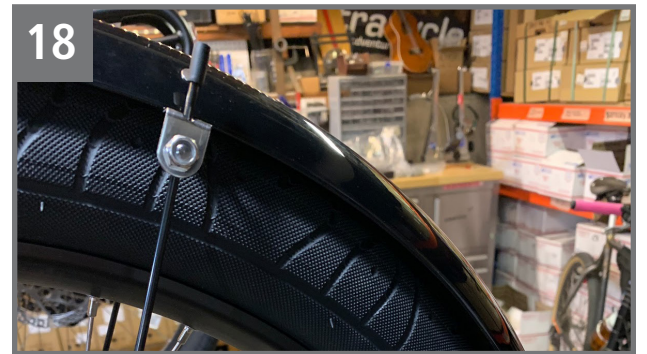
As with the front Fender, trim the excess strut length and cap with the remaining rubber boots.
