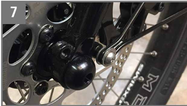
7 When mounting the fender on the caliper side add a spacer between the fork and the fender strut.
