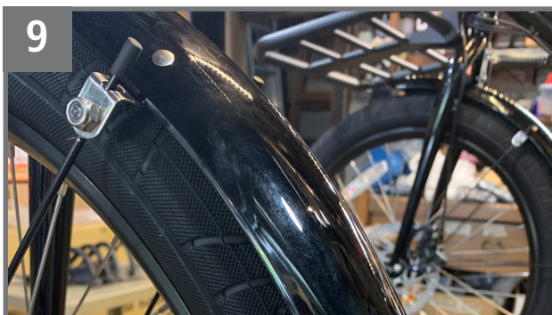
9 Snip off the excess strut length and cap them with the provided rubber boots.
