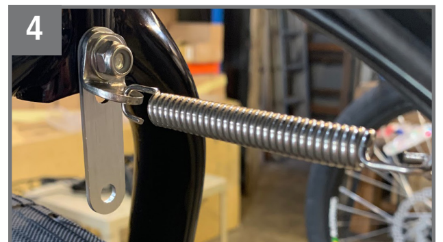
4 With both sets of nut & bolt still loose, assemble the Stabilizer spring.
