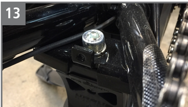
13 If installing the rear Fender while in Sport mode use this mounting point. For rear Fender installation while in Utility mode see steps 14 & 15.
