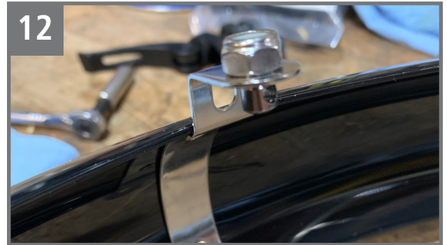
12 Fender eye bolt and nut assembly detail.
