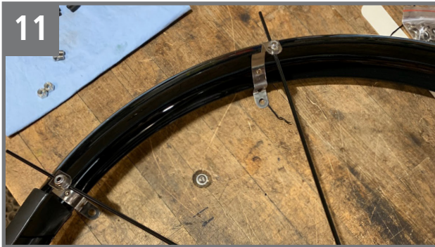
11 Like for the front Fender, it is easier to install the rear Fender struts off the bike.
