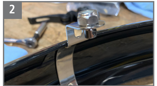
2 Take note of the nut and eye bolt configuration.
