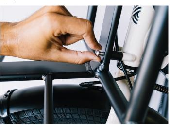
**01 I**Tighten all four bolts smoothly and evenly, alternating in a criss-cross pattern. Tighten the bolts to 6-10 Nm.
