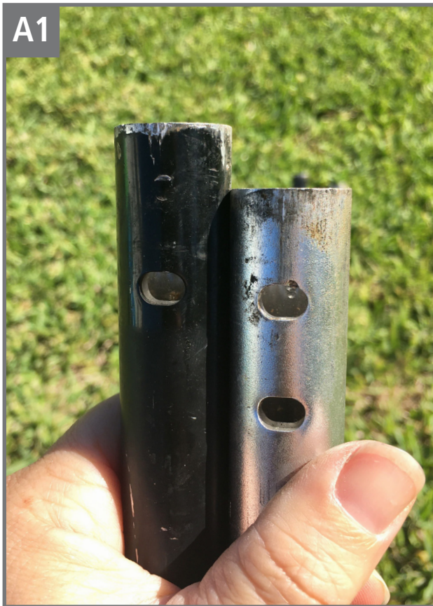
The rear end of the Leap U-Tube (black) has a bolt hole 28mm from the edge of tube. The LT2 U-Tube (silver) has two bolt holes, however the first is too close to the end to allow for a safe minimum insertion into the Leap tailpiece.
