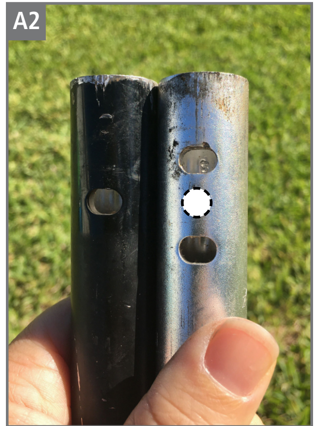
A new hole must be drilled between the two existing holes at 28mm on-center from the end. Secure the U-Tube to a stable work surface and mark your hole location. Using a 1/4" bit, drill your new hole. Be careful to not drill through both sides of the U-Tube.
