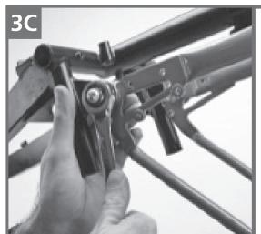
3C: Use a 17mm wrench to tighten both dropout fixing bolts to 30-40 N-m.
