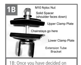
proper placement, assemble the clamping hardware on the longer M10 carriage bolt as shown.
