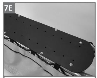
7E: Once all bolts are installed, tighten the bolts to 3-4Nm.
