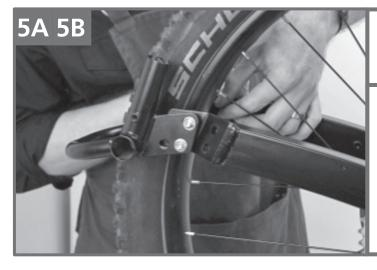
5A: Install the rear wheel in the Leap Frame.
