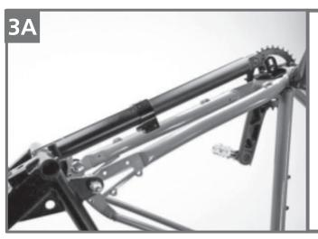
3A: Attach the Leap frame to the bike frame, by inserting the dropout fixing bolts into the rear dropouts of the bicycle as shown.
