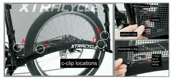
**Step 4a:** Attach 2 vertical c-clips (A + B) to the bottom of the WheelSkirt at the front and rear locations indicated. Make sure the gap in the clip faces out toward you. Vertical locations will have five spaces between ends of clips. The front vertical clip should be located just under the front RackLock. The rear vertical clip will be located just above the back RackLock.
