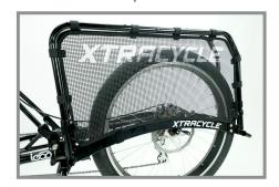
Go back and if necessary, re-tighten all straps until WheelSkirt is firmly tensioned around the rack and LEAP frame. Pressing with your hand toward the wheel with ten pounds force you should not be able to cause the WheelSkirt to touch the tire (this is more difficult to achieve with fatter tires).
