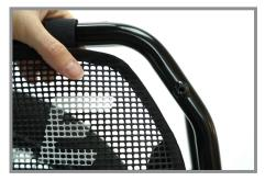
The angle of the WheelSkirt will match the angle of the V-Rack with the Xtracycle logo facing out.
