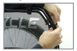
Wrap hook-and-loop straps around vertical uprights (front and rear) of the V-Racks. Pull straps tight before securing.
