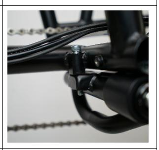
Use a 8mm allen wrench to tighten the M10 Bolt to 18-23 N-m
