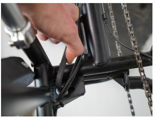
Use a 5mm allen wrench to tighten the M6 bolt to 8-10 N-m
