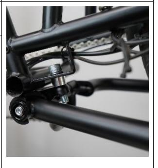
Gently rotate the assembly so the forward mounting threads align with the stabilizing hole next to the boom tube on the Xtracycle frame.
