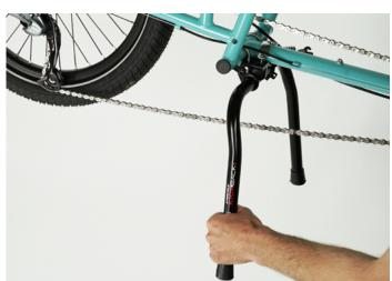
**01 F**Using your 3 mm Allen wrench, tighten the bolts on the BoomStrap or the single bolt below to 3Nm.
