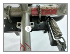
**Step 2a:** Slide the KB3 Radaptor in between the boom tube and the KickBack so that it sits at the front of the mounting plate and cups the boom tube (B).
