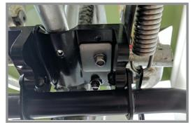
**Step 1a:** With the KickBack legs in the up position, place both Xtracycle BridgeBolts over the Xtracycle's front bridge (A).
