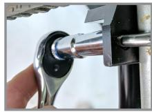
**Step 3d:** Torque all four nuts to 6 Nm.
