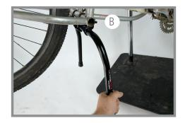
**Step 3a:** Moving the legs as necessary, lightly snug all four nuts with a 10mm socket wrench. Alternating between nuts can keep the KickBack from pulling to one side or the other
