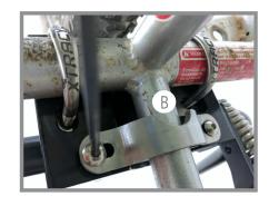
**Step 2b:** Place the BoomStrap over the boom tube (B) and partially thread the two M5 bolts into the KickBack 3 plate. Make it snug, but do not tighten.
