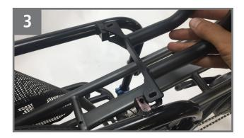
Place the large Hooptie Bracket in the front mounting position. Place the FlightDeck over the Bracket, and loosely re-thread the forward nut & bolt pairs.
