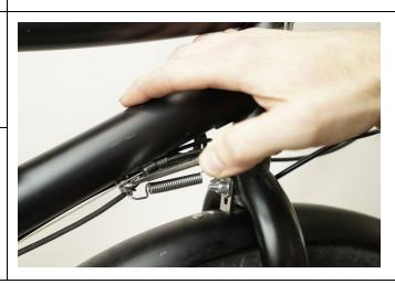
Slip the spring sleeve over the spring to protect it.
