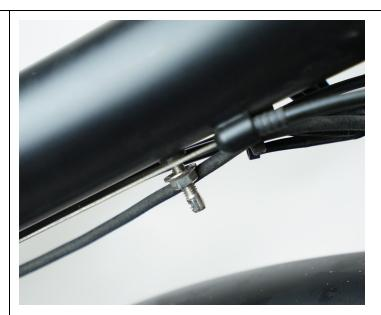
Hook one end of the spring through the small hole on the fork crown bracket.
