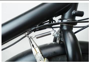
Check to make sure that the eye of the eyebolt is 90 degrees to the axis of the bike.
