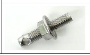
Thread the eyebolt into the boss on the underside of the downtube until the locknut contacts the frame. Leave it loose enough to rotate.
