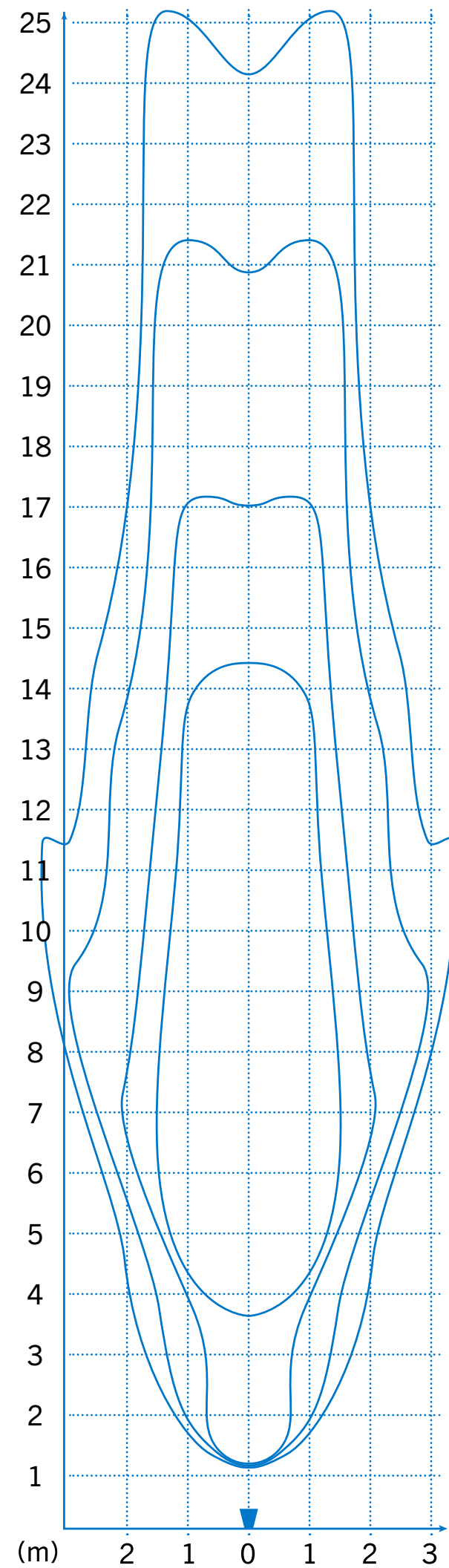
Light spread when H-Black Pro is mounted on top of the front fork of a standard men's bicycle.
