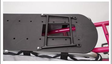
The two larger, longer, bolts (M6x45mm) and washers are used in the foremost two holes, and should pass through the blocks welded to the V-Racks, and Hooptie brackets if installed. They are then secured with a nut.
