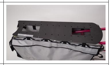
Place the front adapter (flat side down) over the two forward sets of holes, so that the window in the adapter aligns with the window in the deck.
