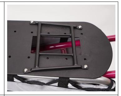
Finish installing the FlightDeck, by replacing the bolts in the two rear sets of holes, as per the FlightDeck LT2 installation instructions.
