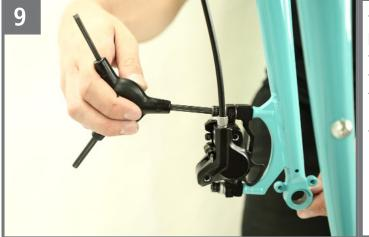
The front brake and its bolts are attached to the handlebars - bolt the brake to the fork per the included Shimano instructions, but do not torque it down yet.
