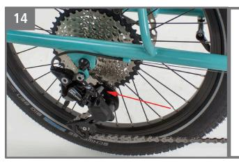
Remember to engage the rear clutch (a grey plastic lever located on the derailleur itself) for better performance.
