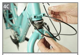
Slide the steerer tube up through the headtube, taking care to make sure the hoses and housing are routed correctly.
