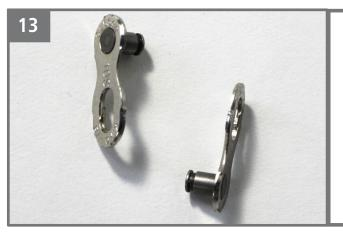
Use the provided KMC Missing Link. Do not resize the chain. It is 162 links on purpose; this will provide the best possible performance.
