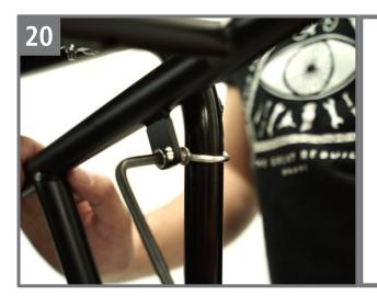
Finally, apply some blue loctite to the threads of the WeddingRings, and tighten them to a more harmonious union - take out the slack, then add a full turn for tension.
