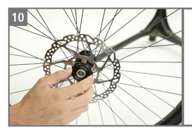
The 180mm front rotor is in the accessory box - attach it to the front wheel using a 16-notch external bottom bracket tool to tighten the center lock nut.
