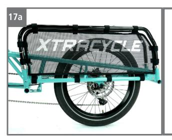
Tighten them enough to keep anything from pushing into the wheel - you may need to loosen the bolts holding the deck on to slip the straps between the deck and V-Racks.
