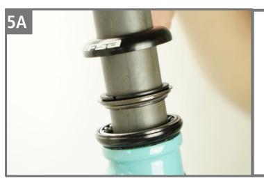
Slide on the upper bearing, top race, split bushing, bearing cap, spacers, and the stem.
