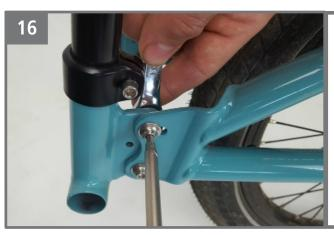
Make sure the tailpiece bolts are tight, use a wrench on the backing nut to keep it from spinning. Torque to 6nm.
