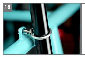
Take some tension off of the WeddingRings to make finishing the deck installation and installing other accessories easier.
