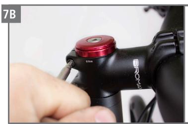
Tighten the stem clamp bolts to 6nM to lock in the adjustment.
