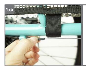
On the lower straps, make sure not to wrap straps around the derailleur cable.
