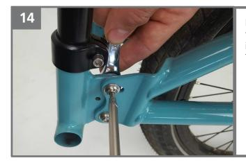
Make sure the tailpiece bolts are tight, use a wrench on the backing nut to keep it from spinning. Torque to 6nm.
