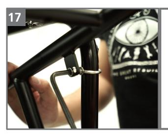
Finally, apply some blue loctite to the threads of the WeddingRings, and tighten them to a more harmonious union - take out the slack, then add a full turn for tension.
