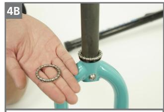
The headset includes a thin rubber seal that sits on the lip of the crown race. Install this first, then the lower bearing (the lower bearing is larger than the upper). Grease liberally.
