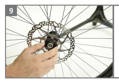
The 180mm front rotor is in the accessory box - attach it to the front wheel, this requires a 16-notch external bottom bracket tool to tighten the center lock nut.
