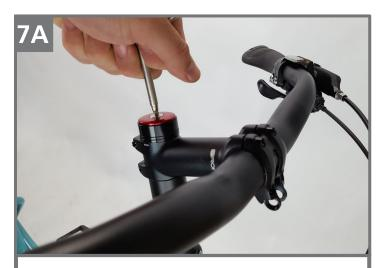
Tension the headset bolt to adjust the headset. You may now release the zip-tie or toe-strap that was holding the fork.
