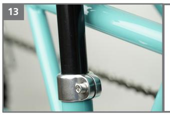
Make sure the RackLocks and V-Racks are seated correctly: The racks should be fully inserted into the uprights and the RackLocks should be pushed all the way down on the uprights and the outer clamp should fully cover the inner collar. Torque all bolts to 5nM.
