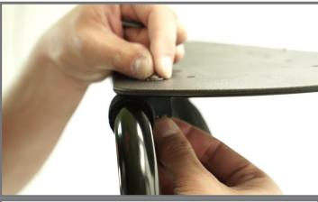
If you've already installed your Hooptie handrails (optional) secure the deck by tightening the four bolts already in the deck and installing the four long bolts and nylock nuts provided into the empty bosses on the V-Rack - two in the front and two in the rear.
