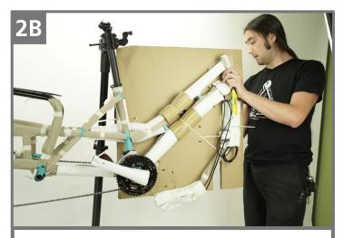
Both the front wheel and the handlebars are attached to the thick, protective cardboard "front wheel block." Remove the bars first and zip tie them to the top tube to avoid damaging the hoses or derailleur cables. Then remove the block and front wheel.
