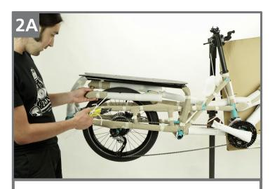
Remove the fork from above the rear wheel - this does not require removing the deck.
