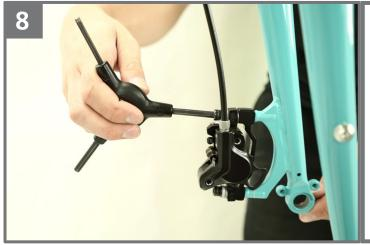
The front brake and its bolts are attached to the handlebars - bolt the brake to the fork per the included shimano instructions, but do not torque it down yet.
