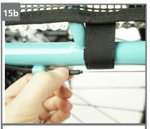
On the lower straps, make sure not to wrap straps around the derailleur cable.
