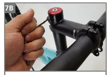
Tighten the stem clamp bolts to 6nM to lock in the adjustment.
