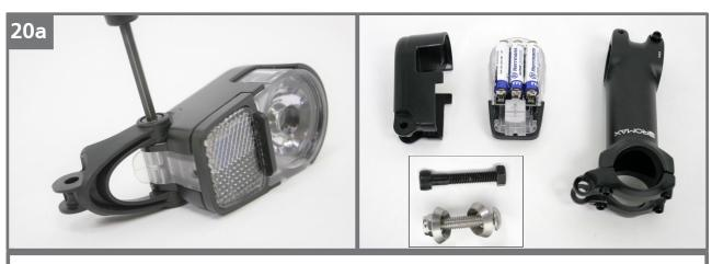
Remove the black nut and bolt holding the light to its bracket. Note that the nut will fit into a hexagonal pocket on one side of the bracket, so you won't need to hold it by hand/wrench.
