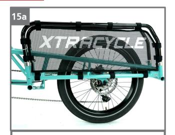
Install the EdgeRunner WheelSkirts, these should be tight enough to keep anything from pushing it into the wheel - you may need to loosen the bolts holding the deck on to slip the straps between the deck and V-Racks.
