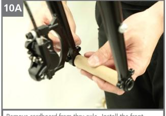
Remove cardboard from thru axle. Install the front wheel, and secure the thru-axle.
