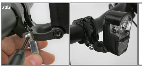
Attach the bracket to the mounting eyelets on the stem using the shorter silver bolt and matching nut. The semi-spherical washers should go on either side of the eyelets, pointing inwards.
