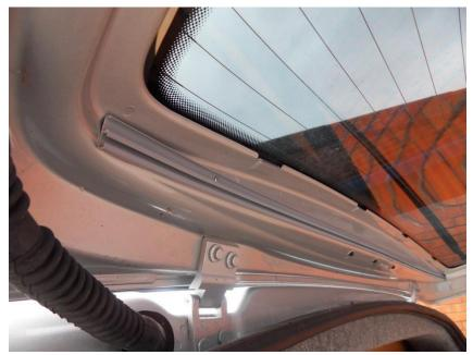
2. The L-Shaped rail fits along the bottom panel below the window for the tailgate door. (Refer to the image below.)
