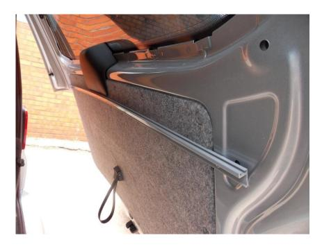
3. Decide where you would like your screws to go and drill the holes accordingly. These holes need to be made in the widest channel of the rail. For the bottom (L-Shaped) rail screws fit on the flat area with the track above ready for the curtains to slide along.
