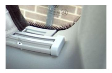
8. Now that the curtains are fitted, look at the end of the curtain with the poppers facing the outer edge as these need to be attached to the side of the window frame. To fit the 6 male poppers please fix where necessary with a rivet or the last remaining 6 screws included in this kit. (Please view the image below for an example how the male poppers on the window frame align with the female poppers off the curtains.)
