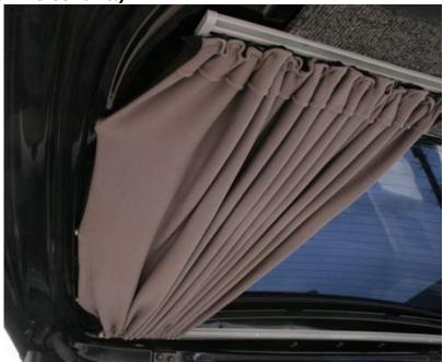
**9.** There are 2 tie-backs supplied within the kit, these are used to attach around the curtains so they stay in place on their own.
