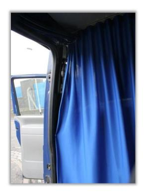
**8.** There are 2 tie-backs supplied within the kit, these are used to attach around the cab divider curtains when they are open. You can use these tie-backs as an option for your cab divider as the curtains will stay in place on their own.
