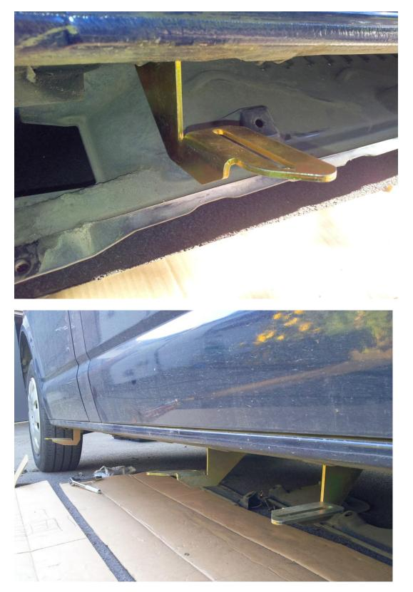
4. Prepare the square-head bolts by inserting them through the grooves under the side step itself. You will need to use 6 of these bolts and position them accordingly to the same width as the brackets being bolted on the side skirt sills done in previous steps (1, 2, and 3).
