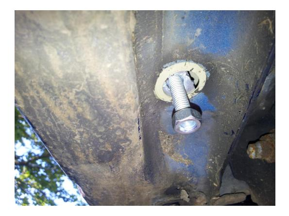
3. Tighten all brackets with the bolts and nuts supplied with the kit. Do this for all the brackets so they are secure under the sills. – Look at all images below for results.
