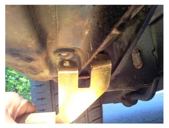
2. Remove the rubber seal and insert the bolts into, ready for them to bolt on the three brackets. - Look at all images below for better viewing.
