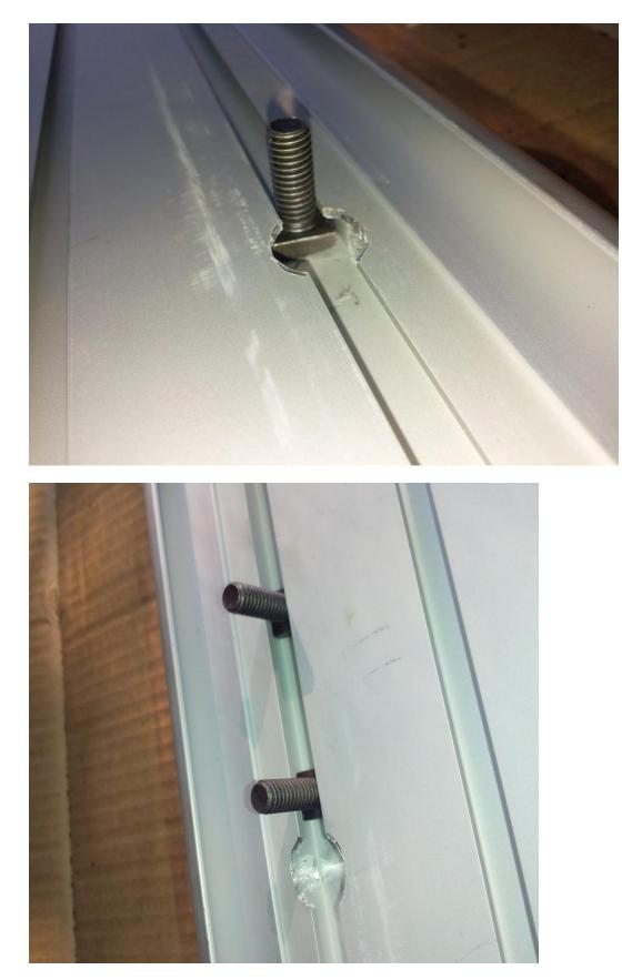
5. Place the side step onto the brackets in position through the grooves. Use 6 nuts to tighten all 6 bolts when fitting the side step. Please ensure it is tightened properly and then test the side step carefully.
