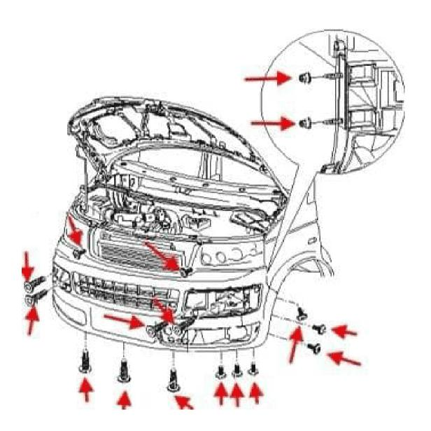
The fixing screws are located in the highlighted areas.
