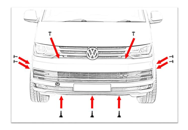
When fitting the T5-X you require to fit the 2 screws on both wings, 1 screw on either side of the headlamp and 3 screws at the bottom underneath.
