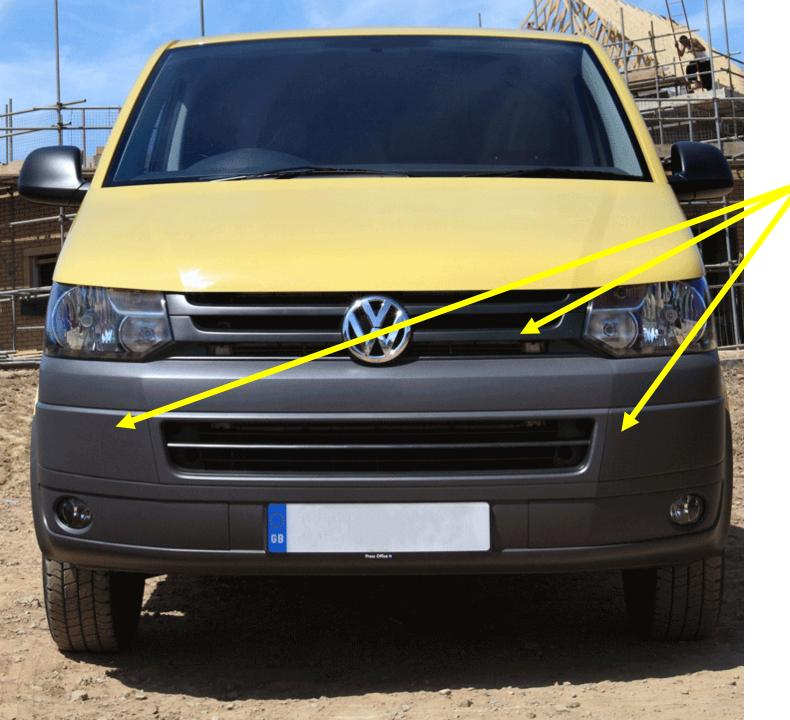
Remove the bumper panels with a panel remover and the main grille to expose the fixing screws.
