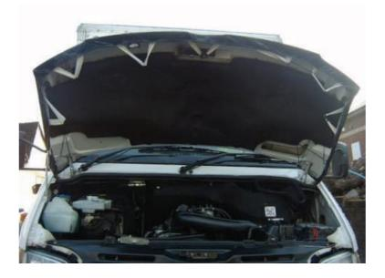
**3.** Tie the bonnet bra using the rope provided, threading the rope through opposite loops, try not to pull too hard.
