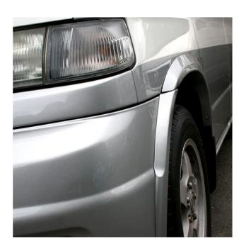
We recommend to bond the wheel arch trims to the vehicle and use a clamp to hold them in place.
