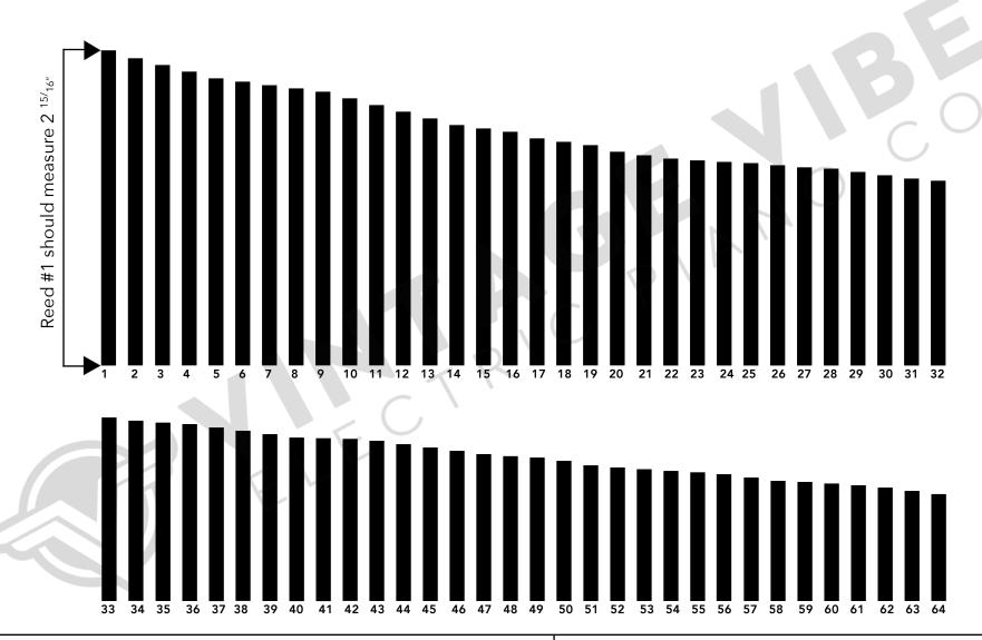
Tools needed: File, Solder, Soldering Iron, Reed Mold, Blank Reeds, Cutter Snips
