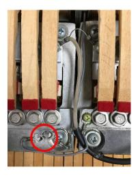
2. Clip coax conductor wire away from terminal lug. Do NOT cut jumper wire.
