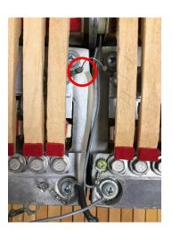
3. Add the new cable's conductor terminal lug to the harp at the same location as the existing jumper wire lug.
