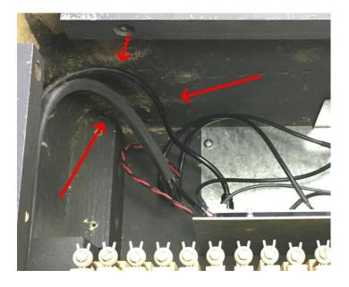
12. Position the lid into place, ensuring that the lid shielding braid wire is making good contact with the lid and temporarily install *ALL* of the lid mounting screws.
