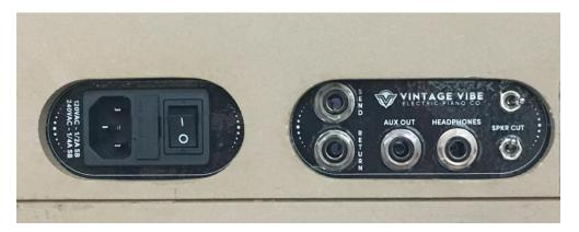
\* We found a good deal of variation in the sizes of the cutouts, the distances between them and their height from the base of the cabinet. We made strides to design the chassis to directly fit as many cabinets as possible; however, it may be necessary to enlarge the cutouts to provide adequate access to all the jacks and switches.
