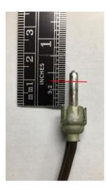
If the pin extends past the shroud by more than 3/8" it may not plug fully into the new amplifier's RCA sockets.
