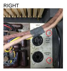
6. Remove the amplifier chassis from the cabinet.
