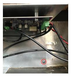
5. Plug the Speaker Cable RCA plug into the corresponding socket on the Jack/Switch PCB (J5).
