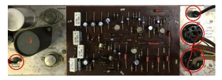
\* If present, you will also need to unplug the "Battery Pack" octal plug from the rear of the instrument. This plug will prevent removing the amplifier chassis.
