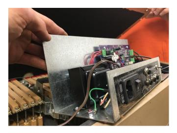
\* Depending on the length of your speaker cable, it may be necessary to unscrew its cable mounting clamp in order to lift the chassis onto the rear of the cabinet.
