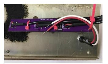
9. Solder the LED wires to the potentiometer PCB.
