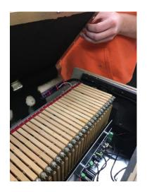
Carefully lift the chassis out of the cabinet to allow access to the trimmer controls. It may be helpful to gently rest the front edge of the chassis on the back lip of the instrument; however, make sure to hold the chassis with one hand at all times.
