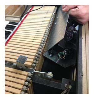
3. Use the artwork on the rear of the chassis to center the chassis within the two rear panel cutouts as much as possible.
