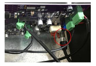
7. Install the included panel mount LED indicator through the lower left hole on the front of the lid and secure it in place with the lockwasher and nut.
