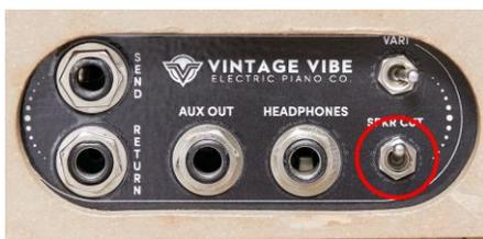
\* The position of this switch has no impact on signal at the headphone jack.
