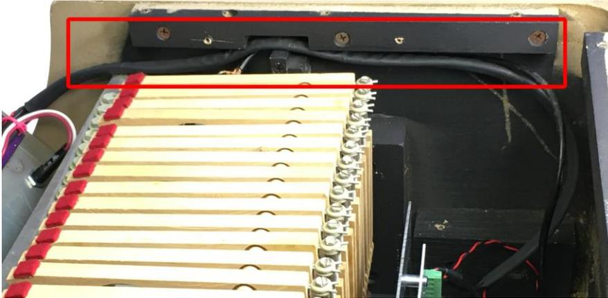
*\* Ensure there is adequate strain relief at the PCB and that the cabling does not interfere with any of the dampers.*
