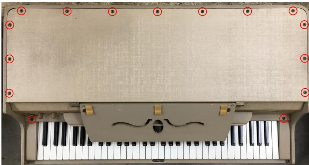
3. Lift the lid from the piano to access the stock amplifier unit.
