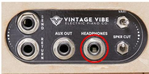
*\*When a pair of stereo headphones are plugged into the Headphone Jack, the output signal to the speakers is cut.*
