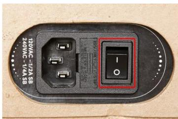
*\* For the least turn-on and turn-off noise, it is recommended to set the Master Volume control fully counter clockwise before turning the unit on or off.*
