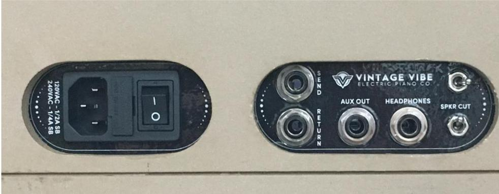
*\* We found a good deal of variation in the sizes of the cutouts, the distances between them and their height from the base of the cabinet. We made strides to design the chassis to directly fit as many cabinets as possible; however, it may be necessary to enlarge the cutouts to provide adequate access to all the jacks and switches.*
