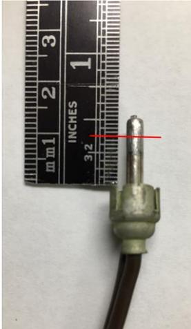
If the pin extends past the shroud by more than 3/8" it may not plug fully into the new amplifier's RCA sockets.
