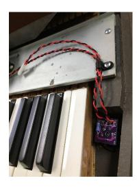
\*This may not be present on all student model pianos. Refer to FX Loop Option section for instructions on installing additional jack plates. When drilling your hole make sure you've provided adequate space for not only the jack plate but also the Headphone Jack PCB to be installed as shown above AND that your hole does not infringe on the leg plate.
