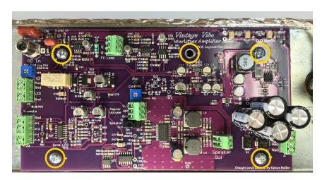
14. Connect Power Transformer secondary wires to PCB connector J1:
