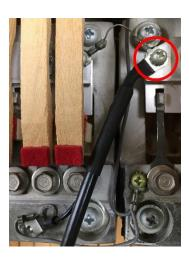
4. Screw down the new cable's shield terminal lug along with the ground jumper lug removed earlier.
