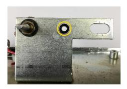
13. Install new Vintage Vibe Wurly Amp PCB on rail using existing screws.
