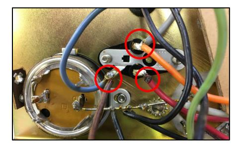
14. Clip out and dispose of the 10W resistor and wires at the positive filter capacitor and rectifier.
