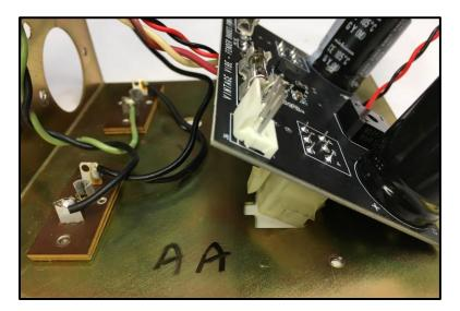
Press the red/white and red/black pairs of wire neatly back against the chassis walls along with the previously dressed green/black pair.
