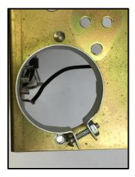
22. Clip all the wires at the 4-Pin DIN or Cinch (pictured) socket.
