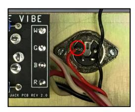
38. Route the black wire from the red/black twisted pair to Pin 4 of the 4-Pin connector; trim, strip and install the wire, but do NOT solder yet.
