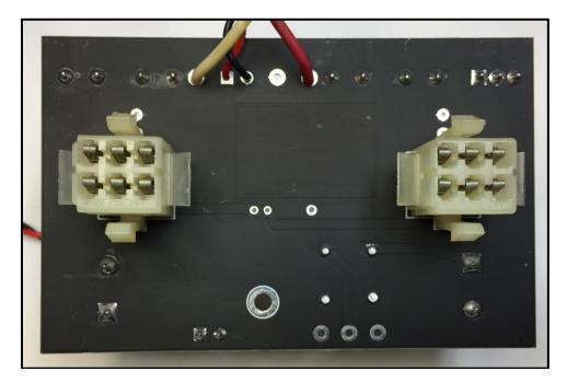
33. Twist the green and black wires as shown. Press them back against the chassis walls and feed them up through the grommet.
