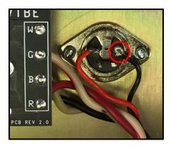
39. Braid the power transformer secondary wires. After braiding, trim to 5" in length from where the wires exit the transformer end bell. Orient the wires so that yellow/red center-tap wire is to one side of both of the red wires as shown.
