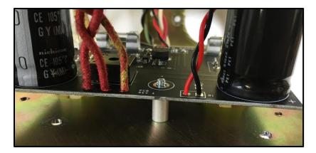
Press down on the PCB to seat the Molex socket connectors to the panel.
