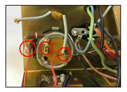
13. Clip the 10W resistor and all four wires from the transistor socket. Dispose of the loose wires.
