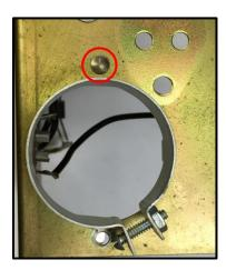
24. With a 1/8" drill bit, drill-out the rivets securing the positive filter capacitor to the chassis, remove and dispose of the capacitor.
