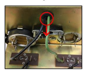
19. Unscrew and remove the TO-3 transistor and socket.
