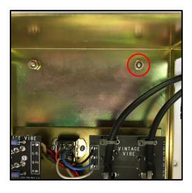
50. Install the included 3/8" wire clamp around the coax cables as shown and secure it in place with the screw and lock nut removed in step 49.
