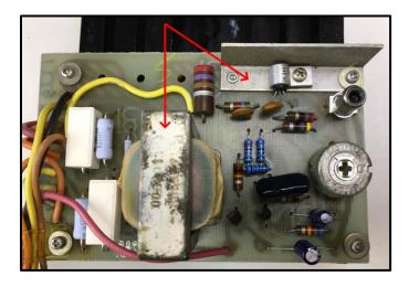
59. Remove the four screws securing the PCB to the heatsink. Set aside the screws, washers, standoffs and nuts.
