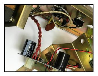
41. Insert the included 7/8" #6-32 machine screw through the rear of the internal chassis panel as shown.
