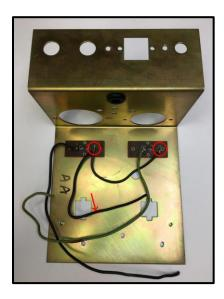
29. Install and rivet the replacement 4-Pin DIN or Cinch socket to the chassis.
