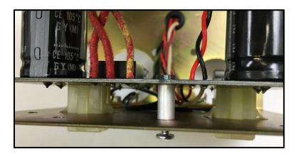
44. Install the included lock washer and hex nut onto the machine screw. Advance the screw until its end is flush with the top of the hex nut. Holding the hex nut against the PCB with a 5/16" nut driver, advance the screw until it is fully seated against the chassis panel, the hex nut is tight against the PCB and the standoff is not able to shift position.
