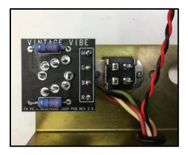
Solder the wires to the PCB pads: "W" = White, "G" = Green, "B" = Black, "R" = Red
