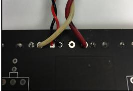
32. Insert Molex socket connectors through bottom side of the PCB. Utilize the silkscreen outline to ensure they are properly oriented.
