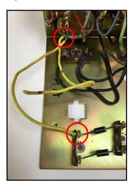
12. Clip out and dispose of the 1.5K resistor, indicator bulb and, if present, "death capacitor".
