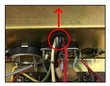
11. Clip and dispose of the wires at both the negative rectifier and the negative filter capacitor.
