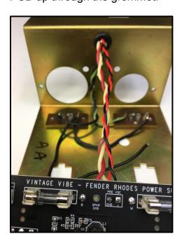
35. Line the power supply PCB up so the Molex socket connectors are sitting directly above the mating cutouts in the chassis panel. Do NOT install them yet.
