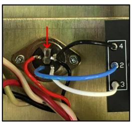
\*\*For units with DIN sockets, do NOT terminate the center chassis tab (indicated above) to any of the solder terminals.
