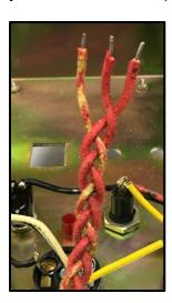
40. Insert the wires through the top side of the power supply PCB and solder. "~" = Red Wire, "CT" = Red/Yellow Wire
