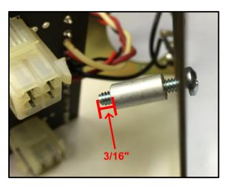
43. Position the power supply PCB so that the Molex socket connectors are in the corresponding cutouts on the internal chassis panel. Position the machine screw to slide the exposed portion through the corresponding mounting hole in the power supply PCB.
