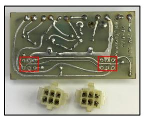
Set the Molex socket connectors aside. The PCB cab be disposed of or kept, as desired.
