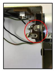
21. Loosen the screw at the negative filter capacitor clamp. Remove and dispose of the capacitor.
