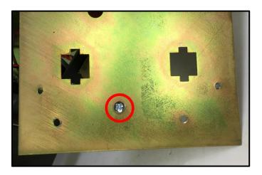
42. Thread the included standoff onto the screw until the screw protrudes through the standoff by about 3/16".
