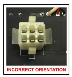
Solder the connectors, ensuring that they are flush to the PCB and do not rotate out of alignment.
