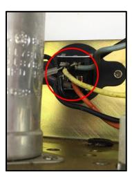
23. With a 1/8" drill bit, drill-out the rivet securing the negative filter capacitor clamp to the chassis, remove and dispose of the clamp.
