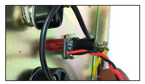
46. Remove the washer and nut from the headphone jack. Using the headphone jack and 4-Pin socket for alignment, place the internal chassis in position within the main power supply enclosure. Reinstall the headphone jack washer and nut.
