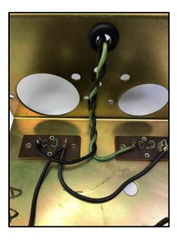
\*Take a moment to inspect the solder connections at the speaker jack terminals. If the wires seem loose, are fraying or the solder joints are not smooth and shiny, re-strip and re-solder.
