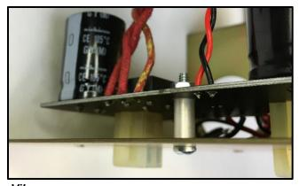
45. Position the internal chassis close to the main power supply enclosure. Insert the LED into the red power indicator lens.
