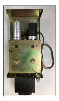
3. With a 1/2" nut driver, remove the nuts securing the three ½" jacks to the front panel. This will allow the internal power supply chassis to be dropped back from the main enclosure.
