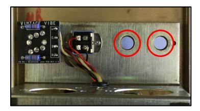
Remove the nuts and washers from the 1/4" jacks on the External Amplifier Jack PCB. Install the jacks through the corresponding mounting holes and install the washers and nuts.
