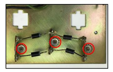
26. With a 1/8" drill bit, drill-out the rivets securing the 4-Pin DIN or Cinch (pictured) socket to the chassis, remove and dispose of the socket.
