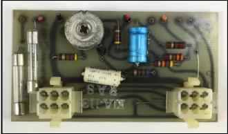
Desolder the Molex socket connectors from the PCB.
