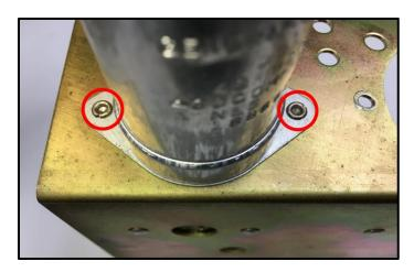
25. With a 1/8" drill bit, drill-out the rivets securing the rectifier terminal strips to the chassis, remove and dispose of the terminal strips and diodes.
