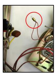
6. Clip the red power transformer secondary wires at the rectifier diode terminal strip and the red/yellow secondary center tap wire at the grounding bus bar. \*Cut the wires close to preserve their length.
