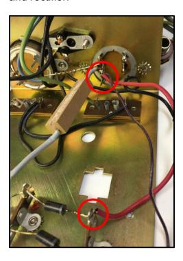
15. Clip the wires at the grounding bus bar. Dispose of the loose wires. Clip out and dispose of the grounding bus bar.
