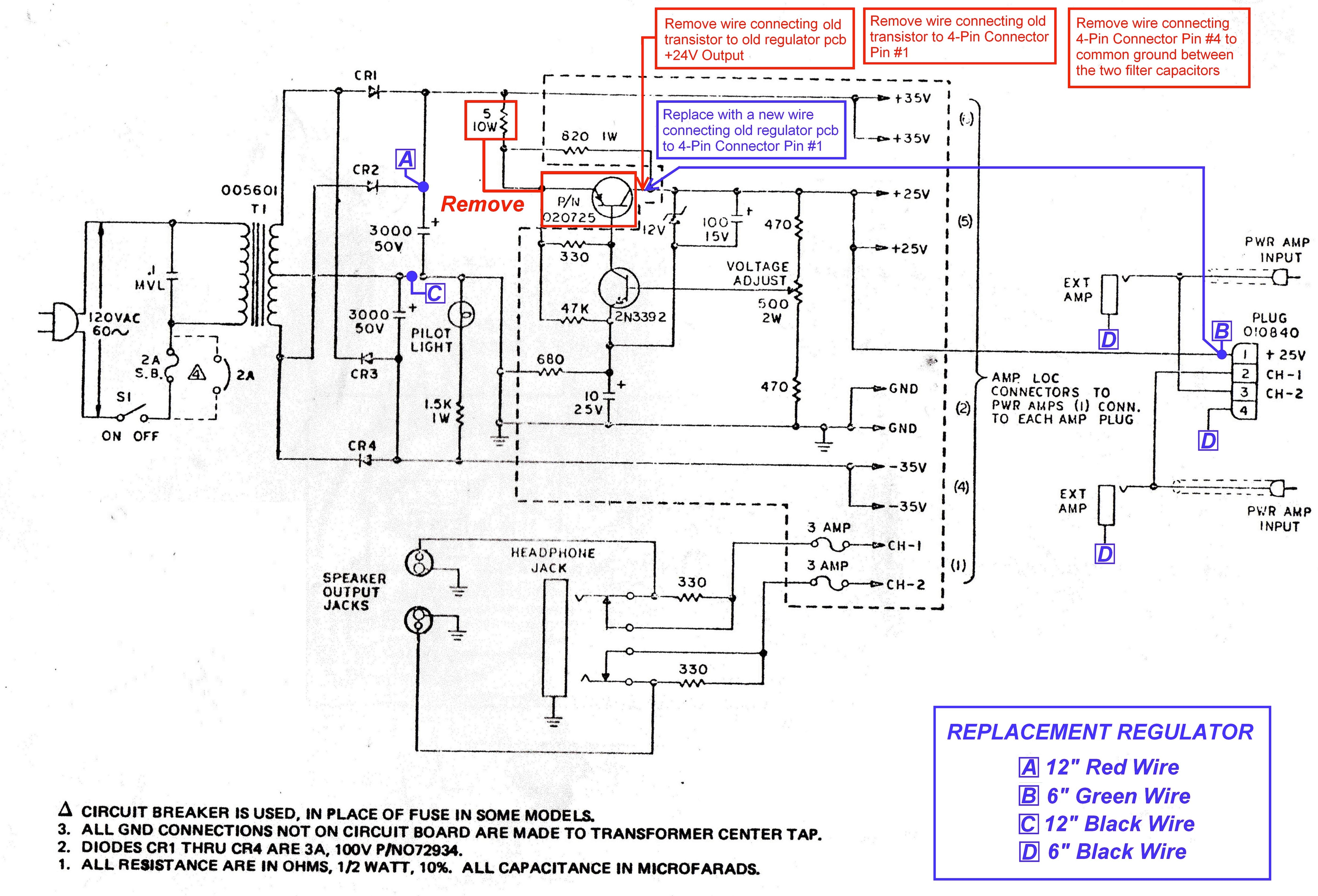
Figure 11-10. Schematic — Power Supply Regulator Assembly (Peterson Design) — 80 Watt Suitcase
