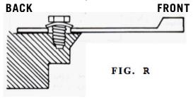
Tuning is accomplished by removing the lead from the reed tip (by filing or scraping a small amount at a time). Continue to remove the excess lead until arriving at the proper pitch. If the reed is flat, the pitch can be raised by removing lead from the tip. If the reed is sharp, the pitch can be lowered by adding lead to the tip or moving the reed as far forward as possible.
