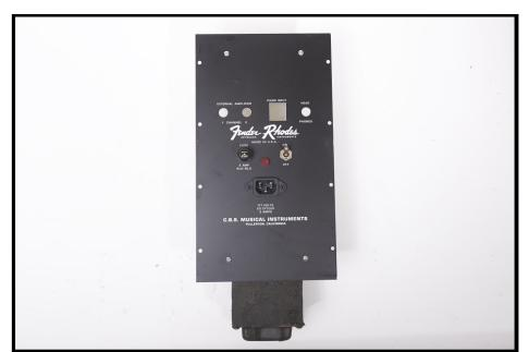
Step #13: Re-install the components into the faceplate / front panel that were removed in step #2.
