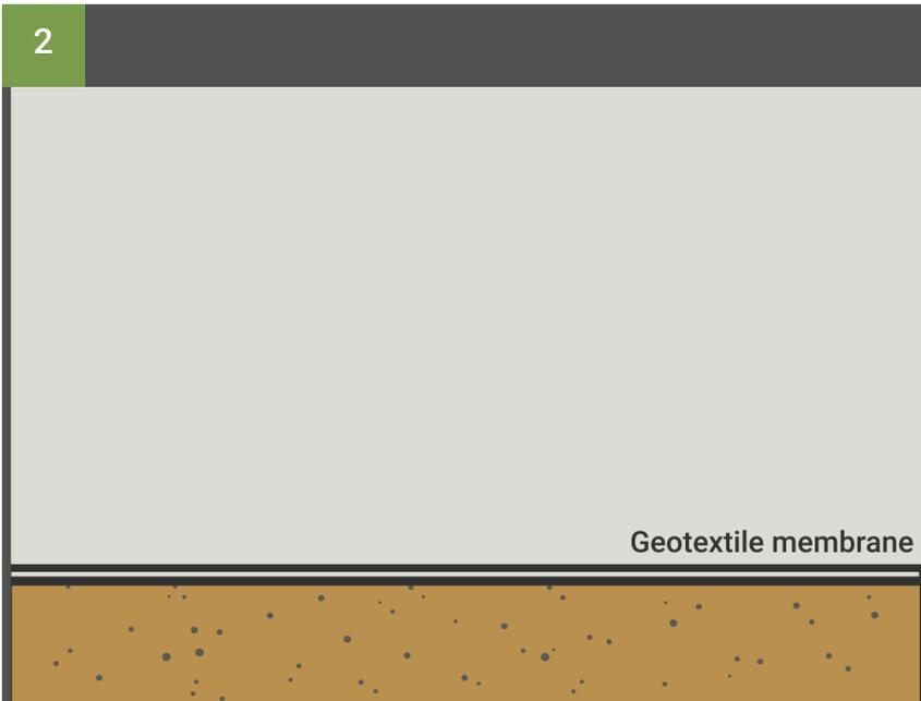
Lay a geotextile membrane. This will help stabilise the base by stopping particle migration of the type 1 into the ground below.
