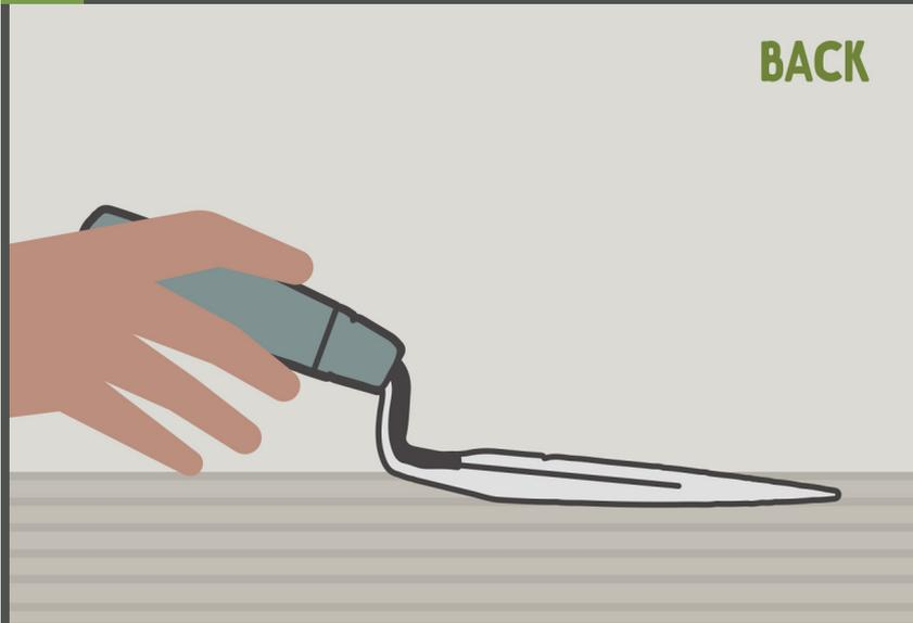
Apply a (approx.) 2mm layer of primer to the back covering of the slab using a trowel. Make sure you get complete coverage on the back, but **DO NOT** get any primer on the front of the slab.
